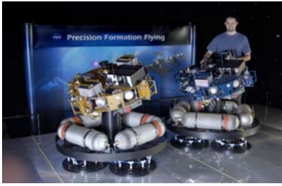
Figure XXX: The 2 robots of the Formation Control Testbed at JPL. Each robot carries cannisters of compressed air to float off a polished metal floor, and a mobile platform (shown tilted). The robots have completed their functional testing and should achieve their operational testing in 2007.
