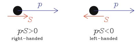
Fig. 4.6 Illustration of lepton helicity. The momentum p is a polar vector, while the spin S is an axial vector, so their dot product is a pseudoscalar, so it changes its sign when inspected in a mirror. The electron from the beta decay of a neutron has  $p \cdot S < 0$  and is referred to as *left-handed*
